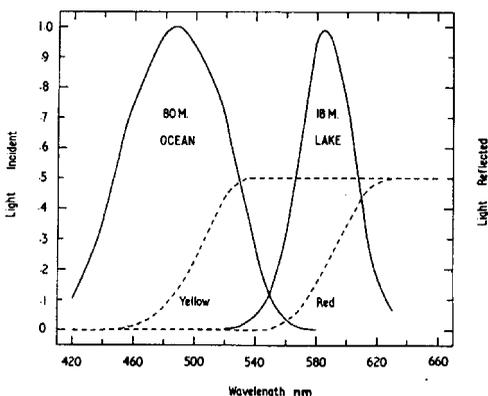
*Typical spectral energy curves for clear oceanic water (Jerlov type III) and water stained with the yellow products of vegetable decay (Jerlov type IX). The depths chosen are those where there remains just sufficient light for colour vision. For comparison are shown idealised spectral reflectance curves for red and yellow objects.*
